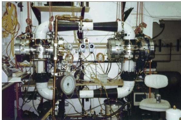
Figure 7. Flow-through standing-wave thermoacoustic refrigerator (Source: Swift, 2002)
