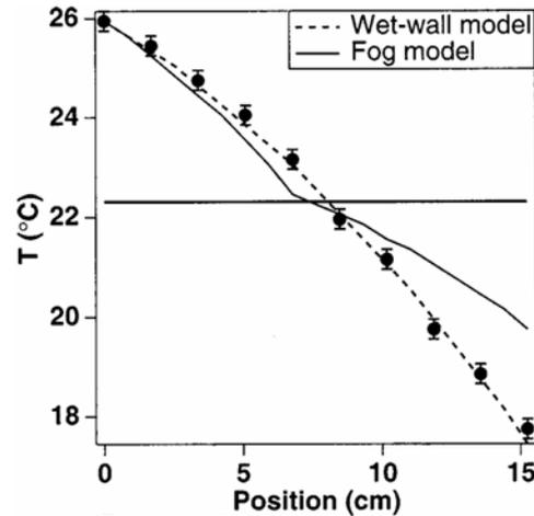
Figure 10. Experimental and numerical results of dehumidifying an air stream with a standing-wave thermoacoustic refrigerator demonstration device (Hiller et al, 2000)
