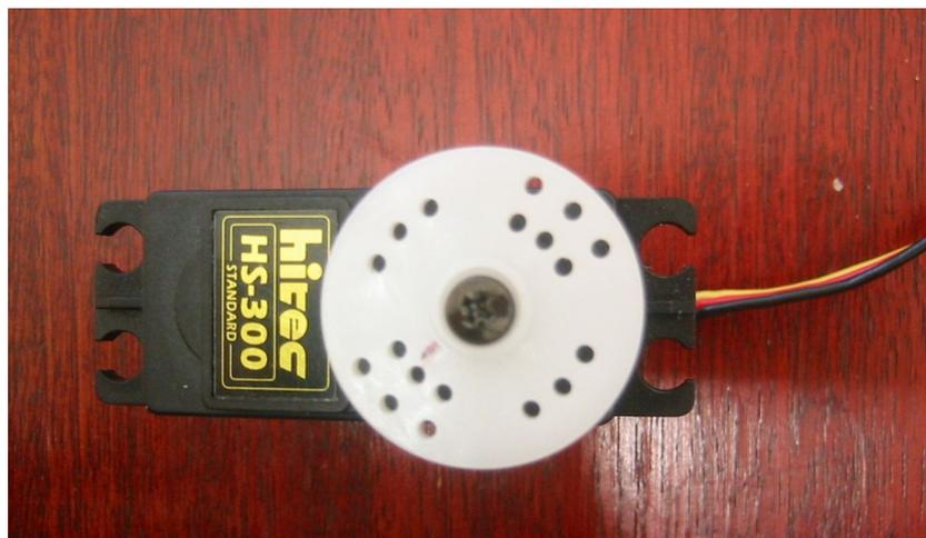
Figure LMP8-2 A small (DC) servo motor
