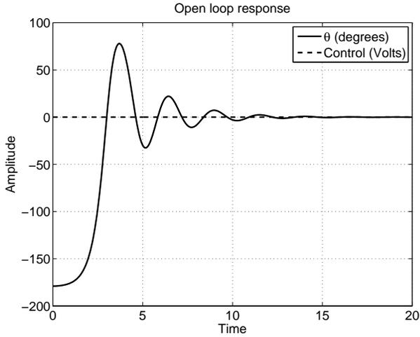
Figure 6: Open loop response when rotated to almost  $180^\circ$  and released
