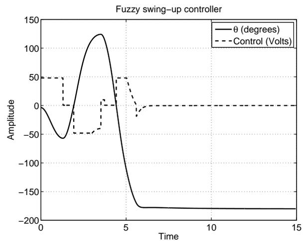
Figure 9: Closed loop response of fuzzy swing-up controller
