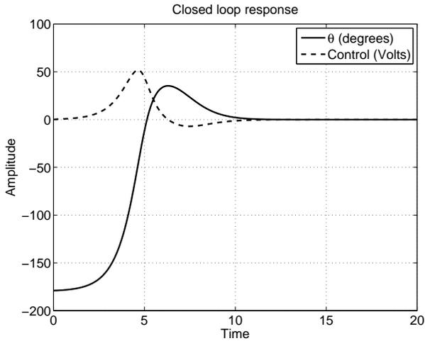
Figure 7: Closed loop response of slosh controller when rotated to almost  $180^\circ$  and released
