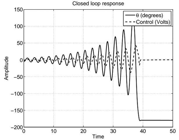
Figure 8: Closed loop response of positive velocity feedback swing-up controller
