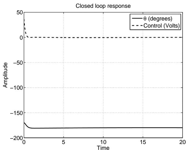
Figure 10: Closed loop response of inversion controller to an initial pose of  $\theta_0 = 170^\circ$
