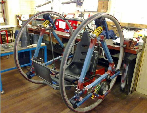
Figure 2: Photograph of the EDWARD diwheel during construction
