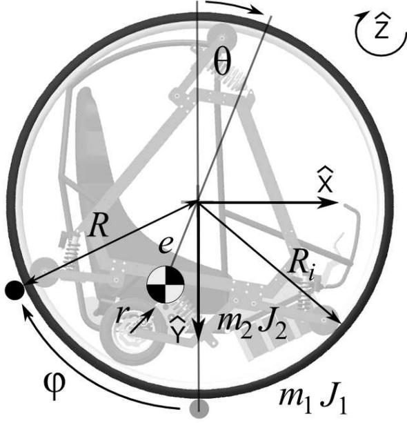
Figure 3: Schematic of a generic diwheel showing coordinate systems, mass distributions and states.
